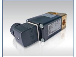
Solenoid valves can be used to actuate on-off valves or implement safety-relevant deactivation for control valves. Pneumatic blocking valves allow the actuating pressure of the actuator to be blocked when the supply air pressure drops below a set threshold value so that the valve remains in its current position.
