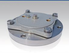
The type 931 pressure transmitter (1:1) can convert the pressure exerted by liquid, highly viscous, or aggressive media into a pneumatic, air signal and transmit this to a pneumatic measuring element controller, for example. The pressure transmitter has a very simple, robust design and requires no maintenance. It is used in any application that requires the pressure of aggressive, very hot, or highly viscous media as well as media containing solids to be measured.
