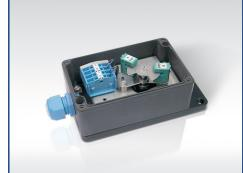
The type 827S signal box is suitable for signalling intermediate or limit positions. It is mounted at the actuator bracket acc. to NAMUR and taps the valve stroke using the patented, zerobacklash ARCAPLUG\* position feedback. Up to three inductive slot initiators are actuated by adjustable switch discs to indicate the current position of the valve.
